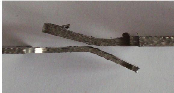
Figure 8 Typical configuration of the tractioned specimen obtained under welding conditions of 2500 rev/min with the welding velocity of 10 mm/min for the slender tool.
